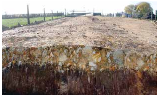
Cross section of compacted StockRock™
